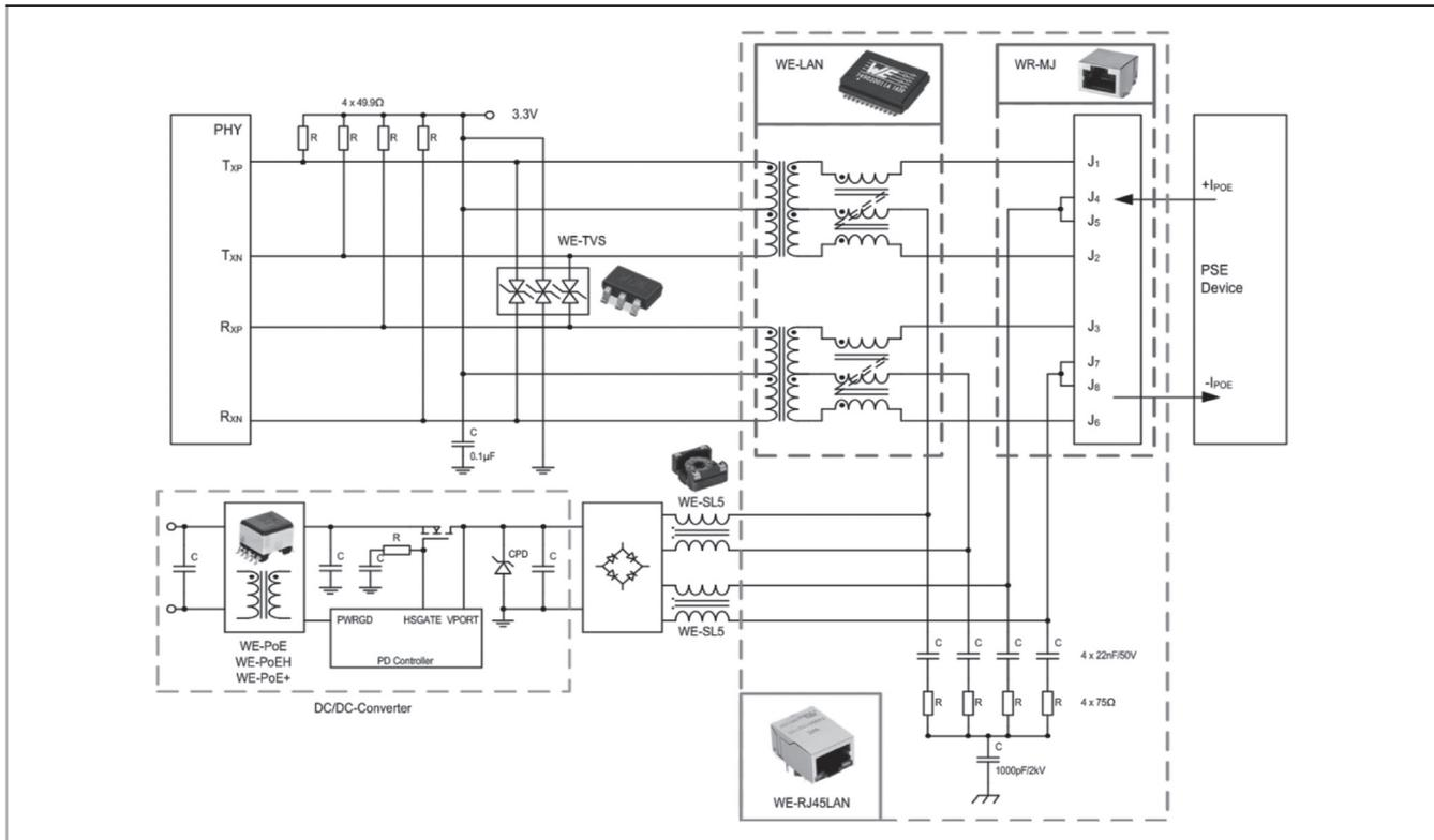
A connection between LAN and Power over Ethernet (PoE) follows the structure as shown in the picture. The Ethernet signals are routed through the cable to the PHY chip whereas the PoE current is transmitted over the same cable and will flow towards the DC/DC converter.
